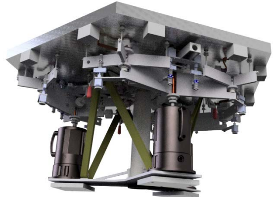
Fig. 5 Conceptual design of the M1 Segment Subunit (Image: ESO)
