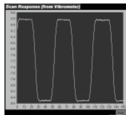
Fig. 11, Mach nullifies the fixture's resonant recoil behavior. The servo parameters are the same as with Fig. 10 (Mach shows equal performance in open loop set-ups!)
