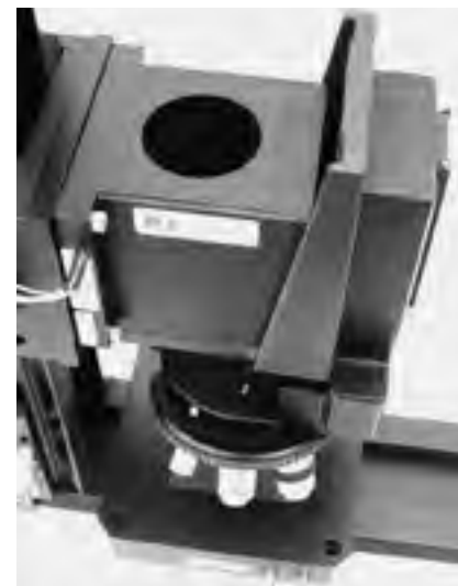
Fig. 3, POWFOC™ Turret-NanoScanner with microscope turret and P-500 XY scanning-stage
