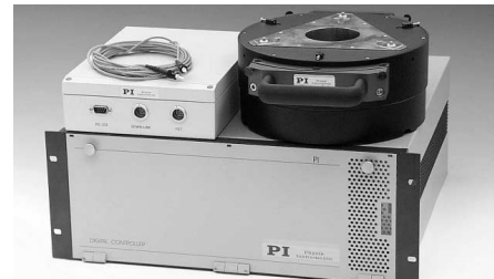
Fig. 5: Fast and compact tilt mirror with capacitive sensors. Tilt range: 2 mrad, resolution: nanorad region. Applications: beam deflection, correcting lens errors and semiconductor technology.
