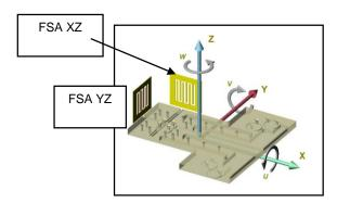
Parameters for *FSA* are the scan axes (linear or angular), scan extent, first-light threshold, and the step size appropriate for the coupling.
