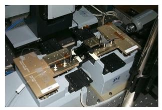
Figure 3. By integrating six degrees of freedom, H-206 facilitates complex alignments like this 10-DOF waveguide MUX/DEMUX packaging.
