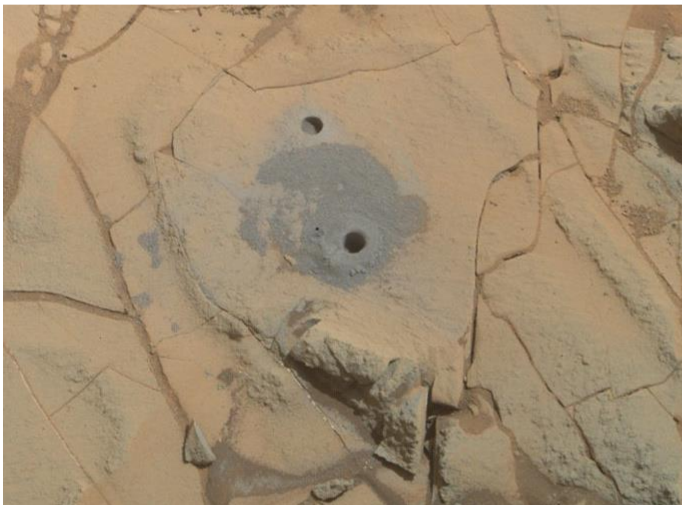
Curiosity's drilling into a target called "Mohave 2" is visible surrounding the sample-collection hole in this January 31, 2015 image from the Rover's MAHLI camera. This site in the "Pahrump Hills" outcrop provided the mission's second drilled sample of Mars' Mount Sharp. (Image: NASA/JPL-Caltech/MSSS)
