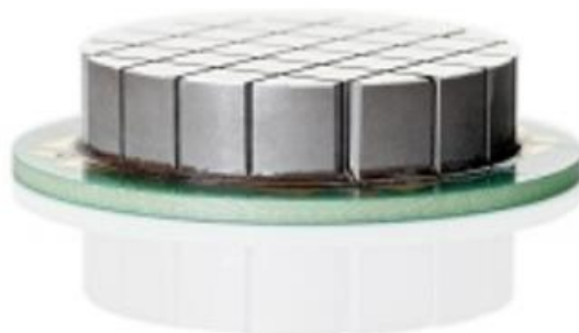
Piezo ceramic in an array structure for generating directed ultrasound (Image: ELAC)
